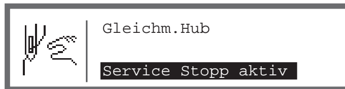
Fig. 3: Calling up the service routine (3)
