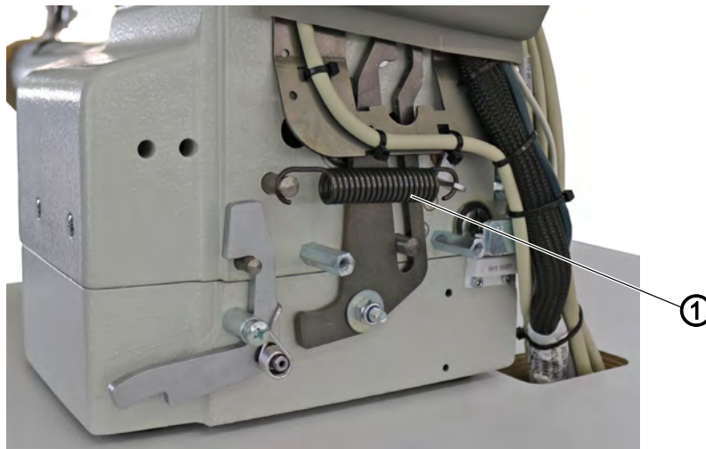
Fig. 19: Setting the mechanical stitch adjustment (1)
