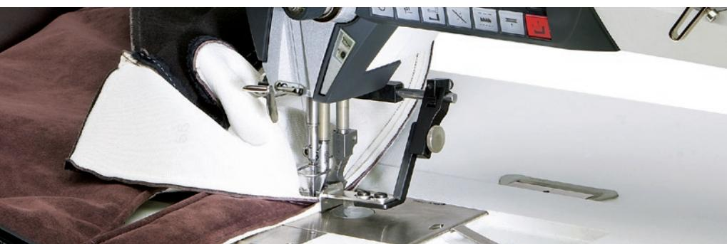
Closing seams/assembly seams during pre-assembly work in the automotive industry
