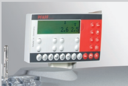
Easy handling of control panel BDFS3 with integrated data reader (SD-card) for transferring sewing programs and machine software
