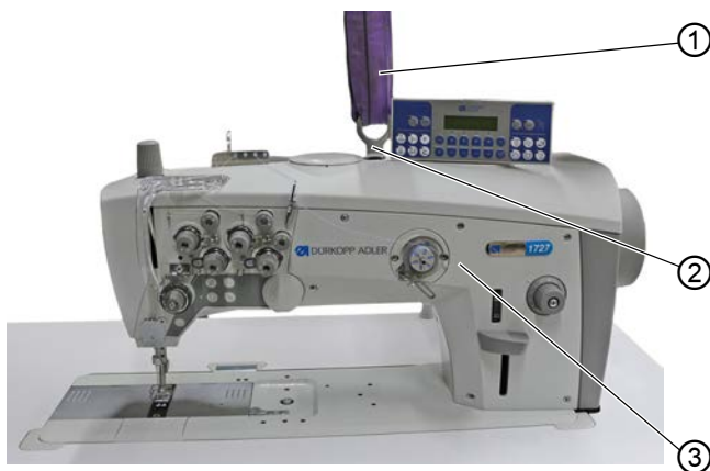
Fig. 39: Inserting the machine head (1)
