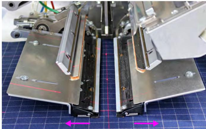
The positions of the transport clamps relative to the folder sole can be set individually and depending on the material in the program. This is made possible by the automatic conversion from double pipe to single pipe and program storage to a wide range of material thicknesses.
