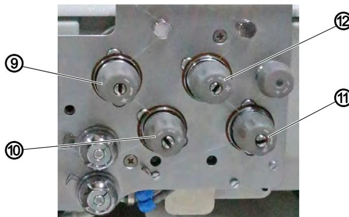
(9) - Additional thread tension - left needle thread
