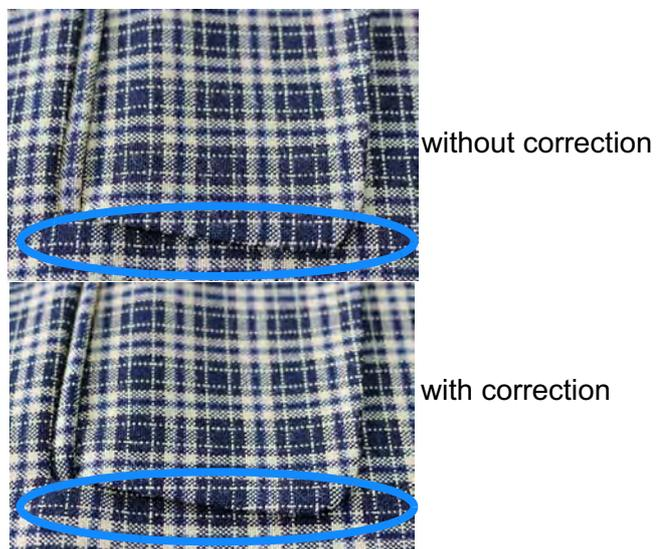
10. If a lateral shift from the pattern is discernible after sewing, this shift can be offset by using stripe correction in the software (
