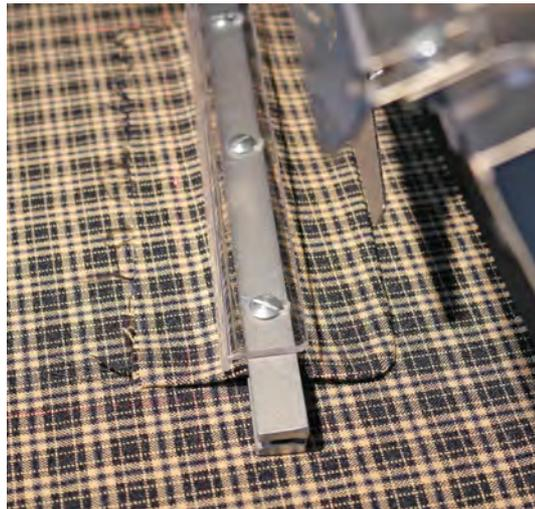
7. Accurately align the jacket front part below the clamped flap as per the pattern.
