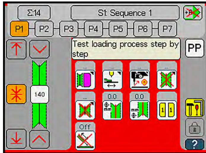
The sewing material is fed through the sewing path without sewing including all functions stored in the seam program. The loading process test is designed to check if the flaps and piping strips are transported correctly through the sewing path.
