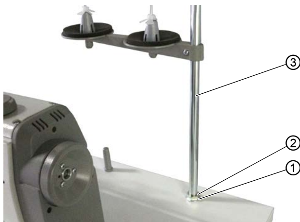
Fig. 71: Assembling the reel stand (1)
