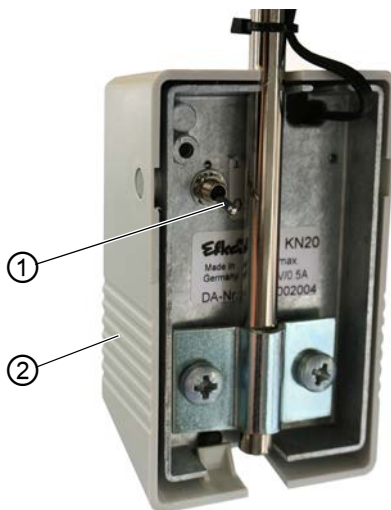
Fig. 33: Using the knee button during sewing (1)
