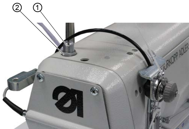
Fig. 32: Setting the sewing foot pressure
