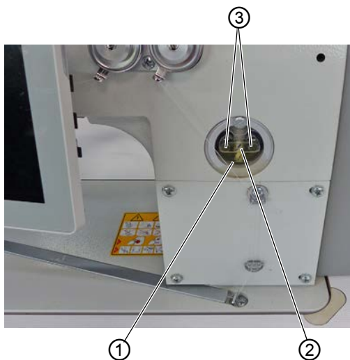
Fig. 64: Checking the lubrication of the machine head
