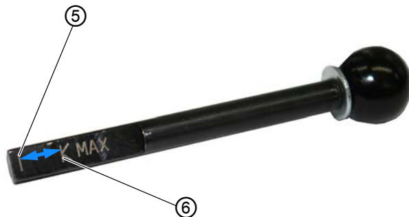
Fig. 67: Checking the hook lubrication (3)
