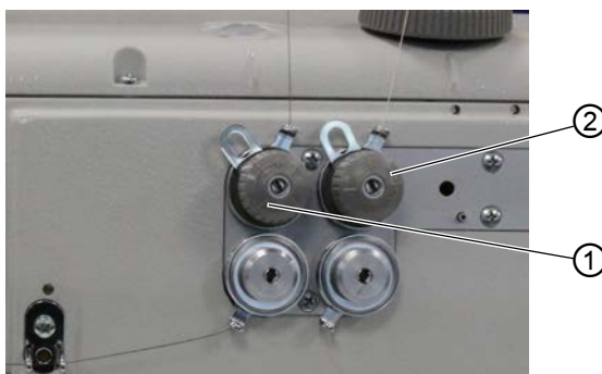
Fig. 23: Setting thread pre-tensioner/tape tensioner (1)
