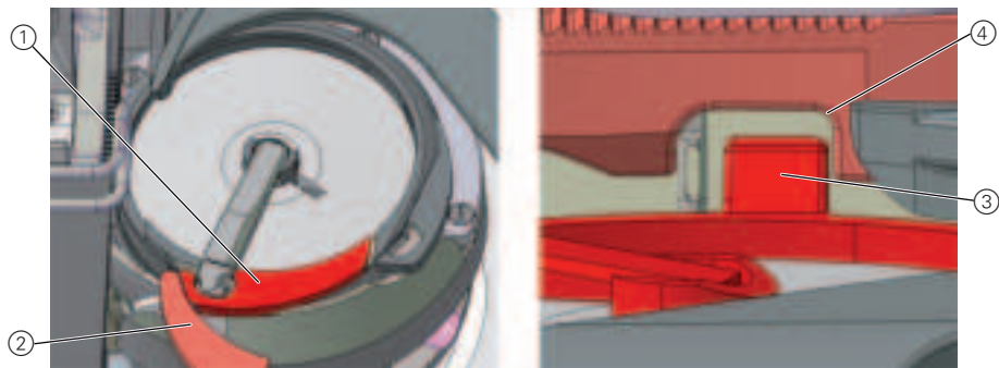
Fig. 47: Adjusting the bobbin case lifter
