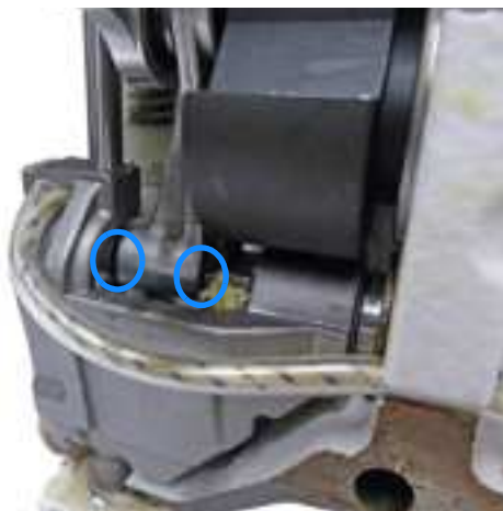
Fig. 39: Aligning the needle bar linkage sideways (3)
