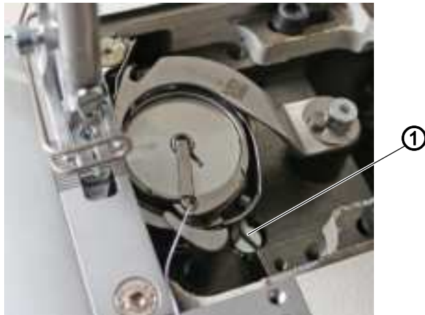
Fig. 97: Checking the hook lubrication
