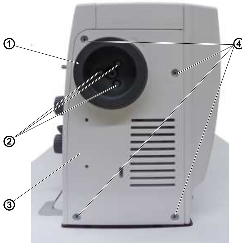
Fig. 9: Disassembling and assembling the toothed belt cover
