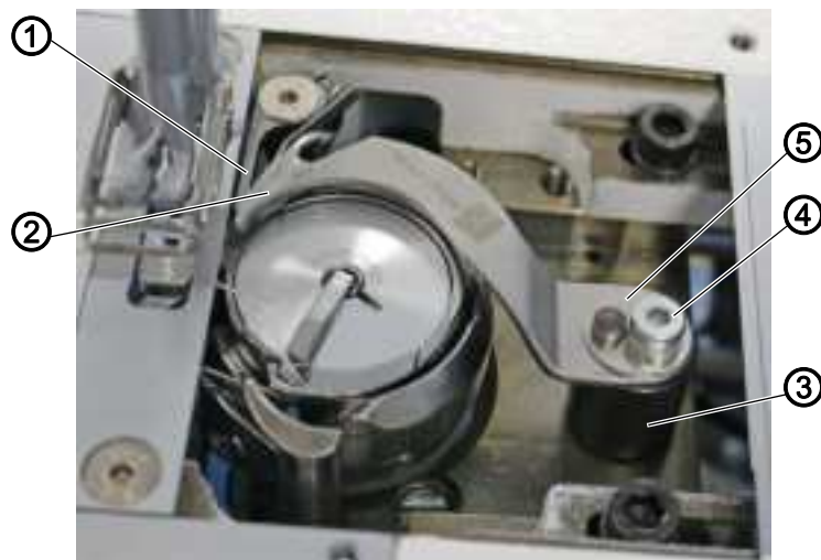
Fig. 64: Adjusting the height of the thread-pulling knife
