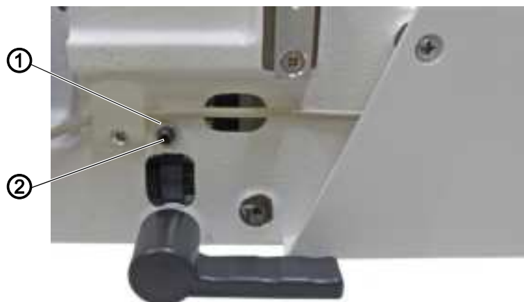
Fig. 55: Adjusting the sewing foot lifting height
