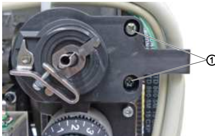
Fig. 57: Disassembling the winder
