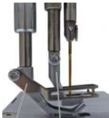
Fig. 53: Adjusting an even sewing foot stroke
