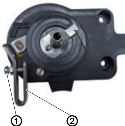
Fig. 59: Setting the winder run and automatic stop (1)
