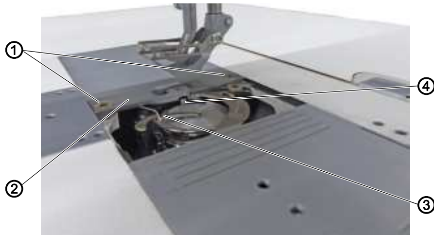
Fig. 11: Disassembling and assembling the throat plate
