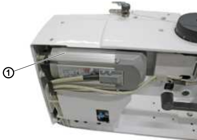
Fig. 94: Cleaning the motor fan mesh (1)
