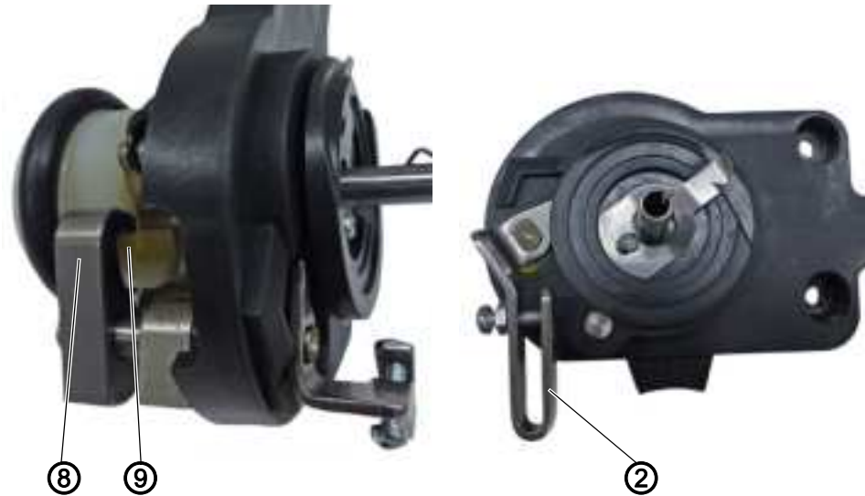
Fig. 60: Setting the winder run and automatic stop (2)
