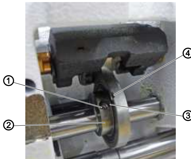
Fig. 52: Adjusting the walking foot movement
