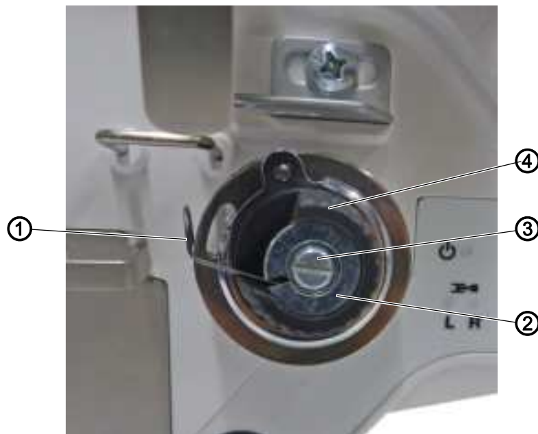
Fig. 56: Adjusting the thread tensioning spring
