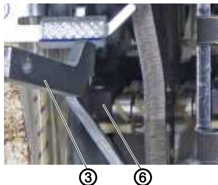
Fig. 25: Adjusting the upper stitch length adjusting wheel (2)
