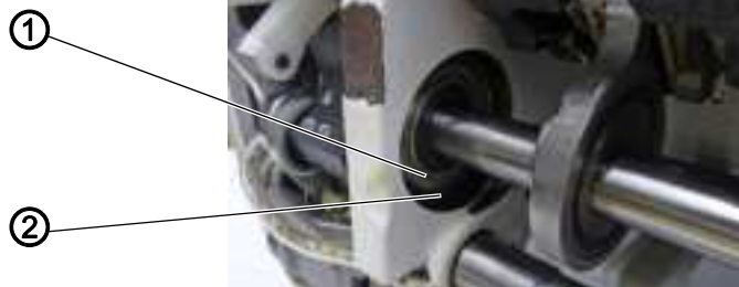
Fig. 17: Positioning the arm shaft crank
