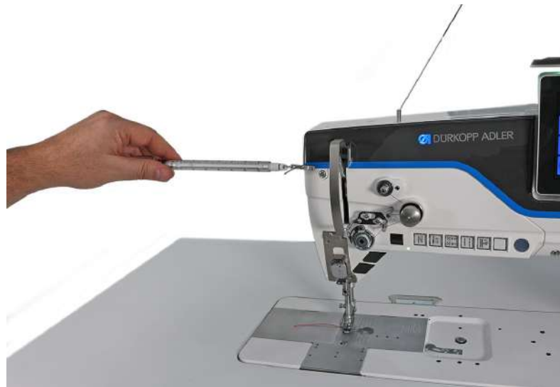
Fig. 129: Calibration of the needle thread tension
